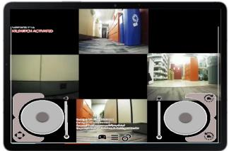
Using a web-based application (OceGo), the user controls the OceBot over a direct socket, or MantaroBot Communications Service link to the OceBot. The OceBot UGV can be controlled from a portable controller, mobile device or a desktop PC. The OceGo web-based controller supports multiple user interfaces including desktop mouse and keyboard, accelerometers and touch screens on mobile devices.
