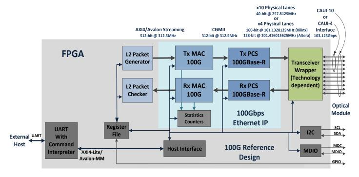
For L1 (physical layer verification and testing) GUI application provides an interface to independently control and configure all 10 10.3125Gbps (for CAUI-10 interface) or 4 25.78125Gbps (for CAUI-4 interface) transceivers used for 100G
