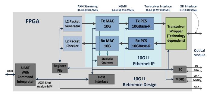
For L1 (physical layer verification and testing) GUI application provides an interface to independently control and configure 10.3125Gbps transceiver used for 10G Ethernet transport. User can configure the transceiver to run various PRBS pattern and configure various transceiver parameters like transmit voltage, transmit pre-emphasis, receive equalization and receive gain.
