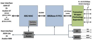
A complete reference design using a synthesizable L2 (MAC level) packet generator/checker is also included to facilitate quick integration of the Ethernet IP in a user design. A GUI application interacts with the reference design's hardware elements through a UART interface (a PCIe option is also available). A basic Linux PCIe driver/API is also provided for memory mapped read/write access to the internal registers with the PCIe interface option. See **Appendix A** for details.
