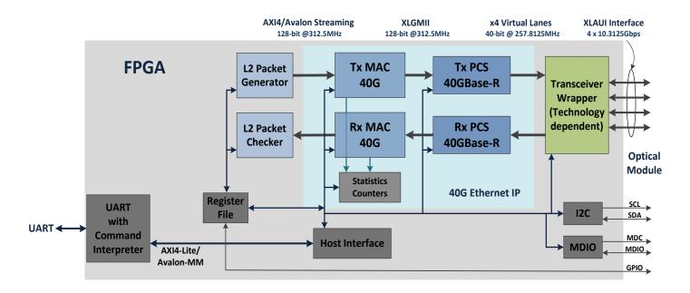
For L1 (physical layer verification and testing) GUI application provides an interface to independently control and configure all 4 10.3125Gbps transceivers used for 40G Ethernet transport. User can configure the transceivers to run various PRBS pattern and configure various transceivers parameters like transmit voltage, transmit pre-emphasis, receive equalization and receive gain.
