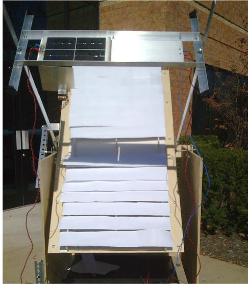
Figure 4 - Solar Tracking Assembly with Mirrors Covered
