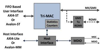
A complete reference design using a simple L2 (MAC level) packet generator/checker is also included to facilitate quick integration of the Ethernet MAC in a user design. An example design and top level wrapper is provided to connect the Tri-MAC core to the popular Marvell 88E1111 Ethernet PHY.
